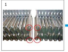
5. Fasten each leg to bottom bracket with M10x50 bolt & M10 nut.
