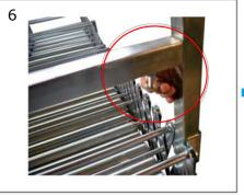
10. Turn conveyor upright & attach stopper assembly to end of conveyor.
